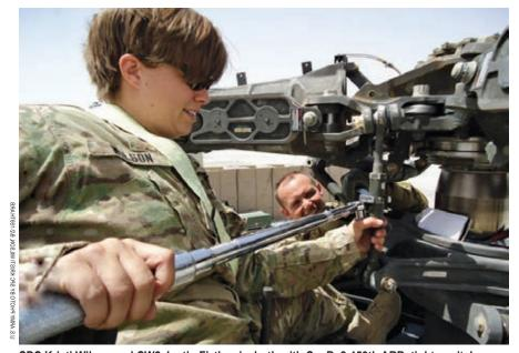
SPC Kristi Wilson and CW2 Justin Fiztharris, both with Co. B, 2-159th ARB, tighten pitch control links during a pre-flight inspection.
