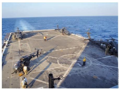
An example of flight deck spotting with ARSOA aircraft on an LPD-class ship.
