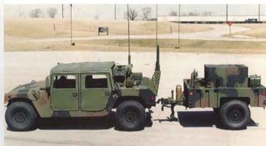
The Tactical Terminal Control System provides initial air traffic services at remote landing sites.
