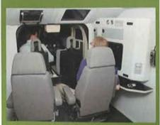
The interior of a TH-67 OFT is spacious and comfortable, with a computer console (on right wall) and overhead screens provide the instructor pilot, students and observers with autonomous ability to program, conduct and playback training.
