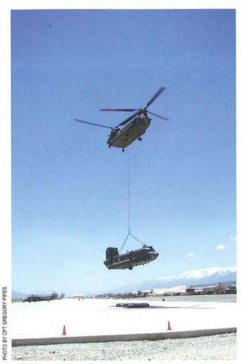
Back home again, the recovered Chinook is carefully lowered to a specially prepared landing pad of 72 wooden pallets and 20 mattresses, to support and limit additional damage to the aircraft.
