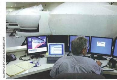
A contractor in his birds-eye perch high up in a simulation bay monitors five TH-67 Creek Operational Flight Trainers which are full-motion virtual simulators.
