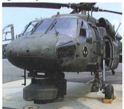
Figure 1: The ALERT external turret-mounted sensor housing.
