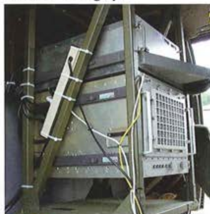
Figure 3: The ALERT's aided target detection and classification processor.
