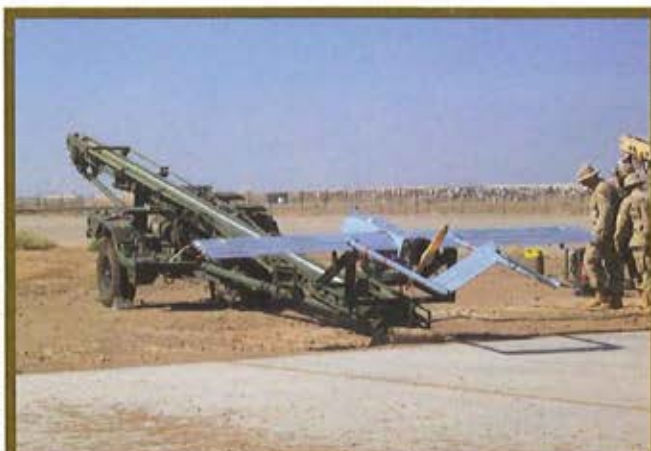
Ready for takeoff, the 328-pound Shadow UAV uses a catapult-type hydraulic rail to quickly launch. Once airborne it can operate at altitudes up to 15,000 feet with a five-hour endurance.
