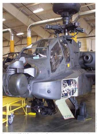
View of AN/APR-39 Radar Warning Receiver sensors installed on the front of an AH-64.
