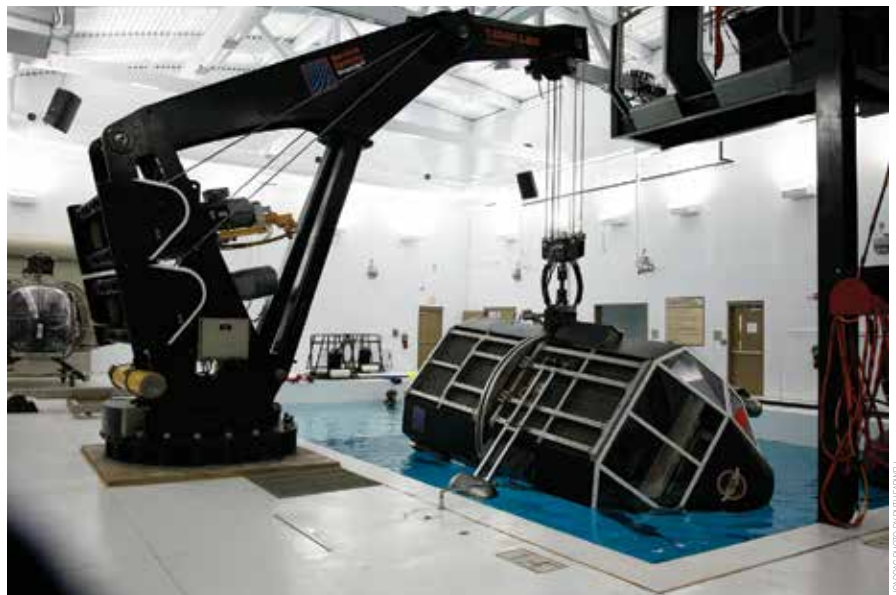
The Modular Egress Training System (METS™) can be configured to simulate any 160th SOAR (A) aircraft.
