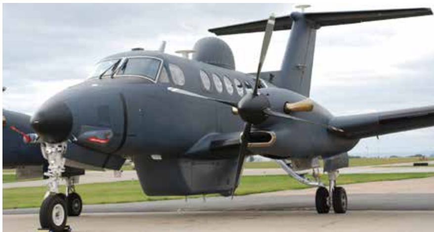
The Medium Altitude Reconnaissance and Surveillance System (MARSS) aircraft is a Quick Reaction Capability, outfitted with electro-optical, infrared, and SIGINT sensors along with an array of communications equipment to process and disseminate the information collected by the platform's sensors to numerous users.
