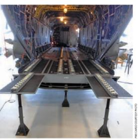
CH 47 with the Cargo On/Off Loading System (COOLS) set up for cargo operations.
