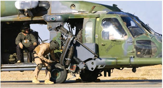
A member of the U.S. Air Force 66th Expeditionary Rescue Squadron checking over the .50 caliber machine gun on the CFD External Gun Mount System (EGMS) prior to flying to a firing range for practice.
