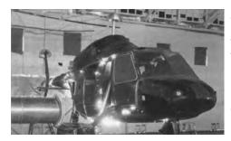
composite material. The Boeing Military Airplane Company's Atmospheric Electricity Hazards Protection Program utilizes a simulator able to produce 200,000 amperes at 1.6 million volts.
