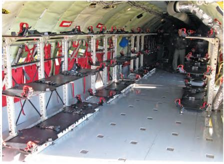
The LifePort Stanchion Litter System (SLS) is available through the Electronic Catalog (ECAT).
