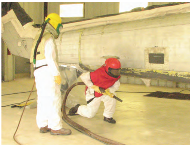
Aircraft refinishing specialists at Lowe's paint facility, work on blasting the paint off a UH-60A.
