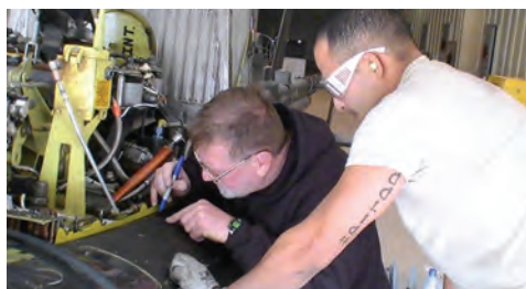
TASMG employees conduct a detailed airframe inspection using non-destructive testing techniques.
