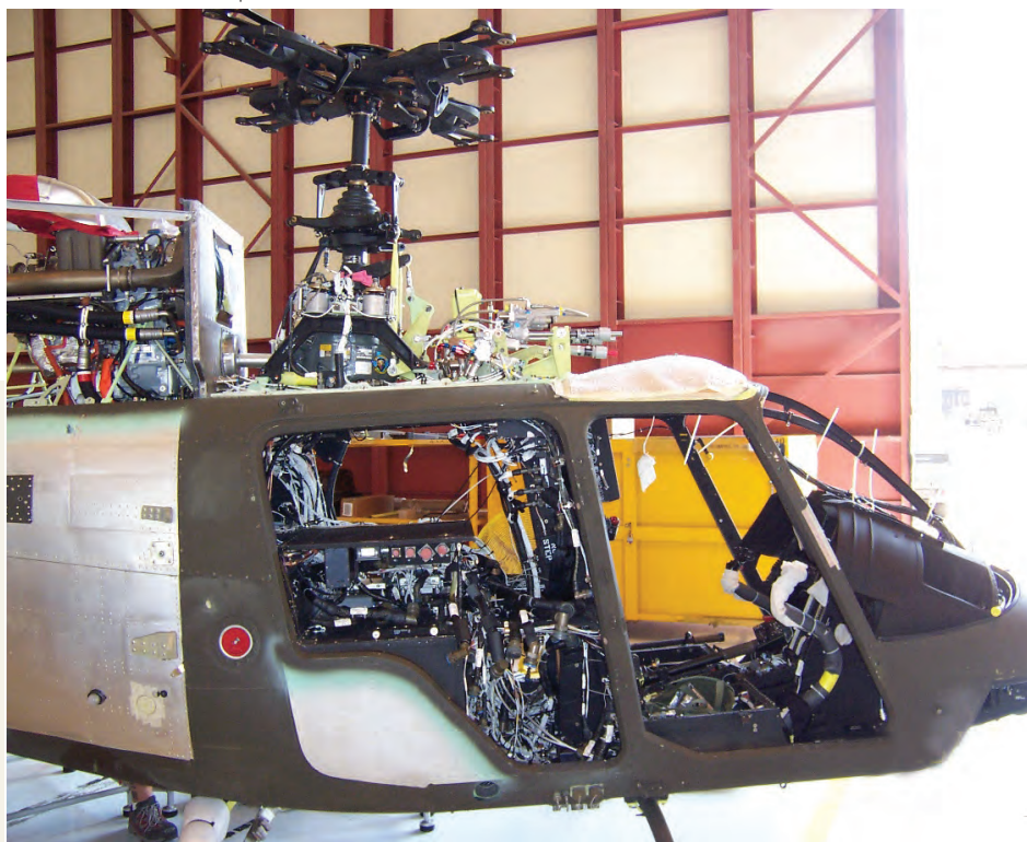
CCAD's first Wartime Replacement Program OH-58D Kiowa Warrior, nearing completion.
