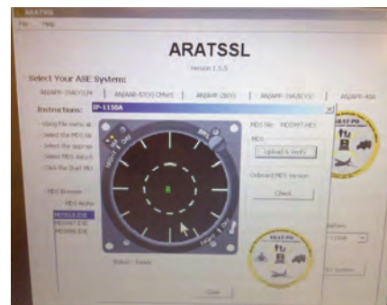
Performing software reprogramming via ARAT supplied MLV kit.
