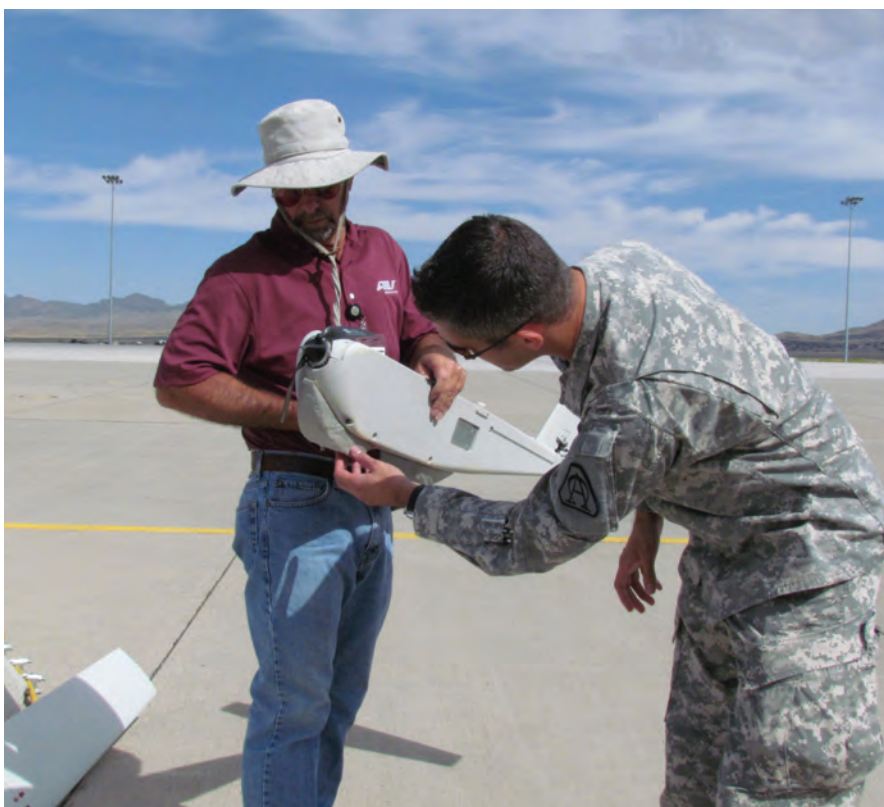
MAJ Jeff Poquette, the assistant product manager for Small Unmanned Aircraft Systems, looks over the condition of the Puma held by contractor Mike Reagan after a landing where the unmanned aircraft seemingly crashes and falls apart. In actuality, it was designed for a sudden vertical drop with parts that are easily put back together.
