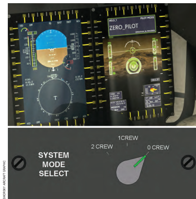
Here in this artist's concept illustration, an optionally piloted vehicle would have a type of selector switch in the cockpit which would allow either a crew, single pilot or a remote operator to control the aircraft. The selected option appears on the multi-functional display above.
