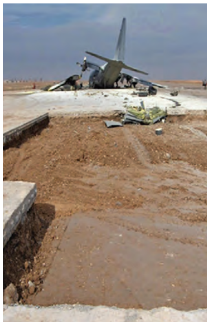
A U.S. Air Force MC-130 Combat Talon aircraft was destroyed Dec. 30, 2004 when it landed on a runway at an Army airfield and encountered a 30-by-30 foot hole in the pavement which was created by ongoing repair operations.
