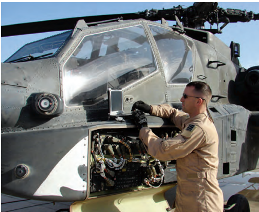
Downloading data from the Modernized Signal Processing Unit (MSPU) on an Apache.
