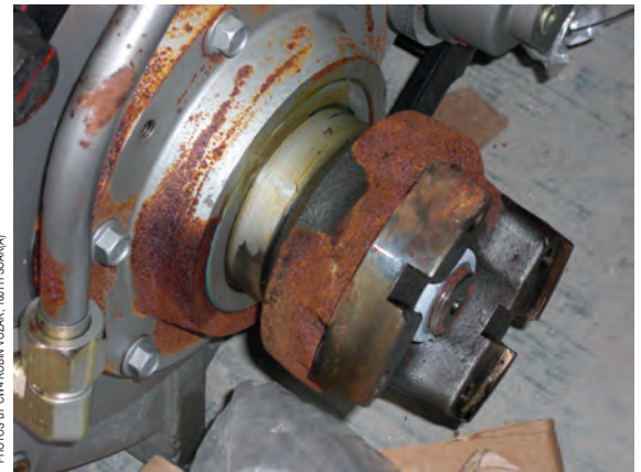
A high speed dynamic helicopter component that has been damaged beyond repair by humidity and environmental conditions.
