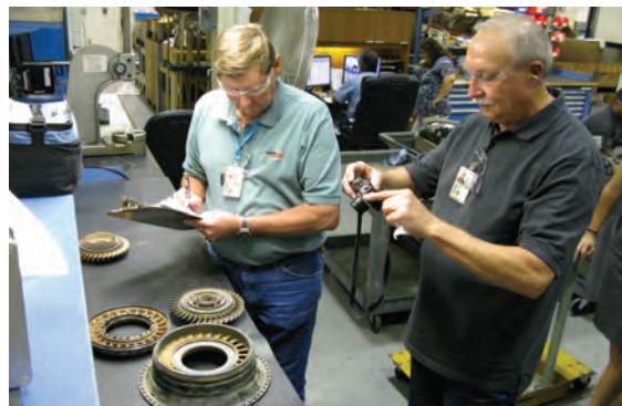
Reliability Improvement through Failure Identification and Reporting program (RIMFIRE) inspectors perform over the shoulder tear down analysis at the depot during the overhaul process, recording critical failure information.
