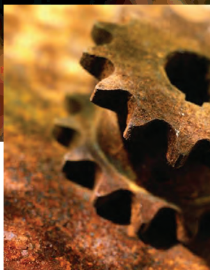
Typical advanced stages of corrosion on equipment like this cog.
