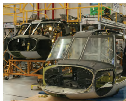
UH-60L artisans replace the nose section of the helicopter during recap at the Corpus Christi Army Depot. The new section is being attached to helicopter.
