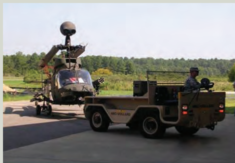
An OH-58D being moved by the SATS during testing at Ft. Eustis.
