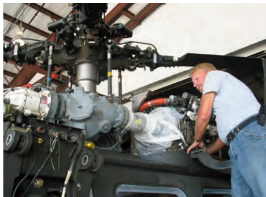
The output shaft gimbal of a UH-60 is inspected during reassembly of the aircraft.
