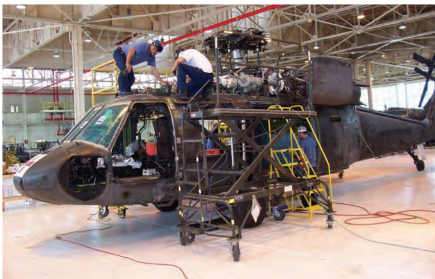
A UH-60 Blackhawk helicopter undergoes Reset. The aircraft is made fully mission capable after having been disassembled to the airframe where inspections and repairs are made.
