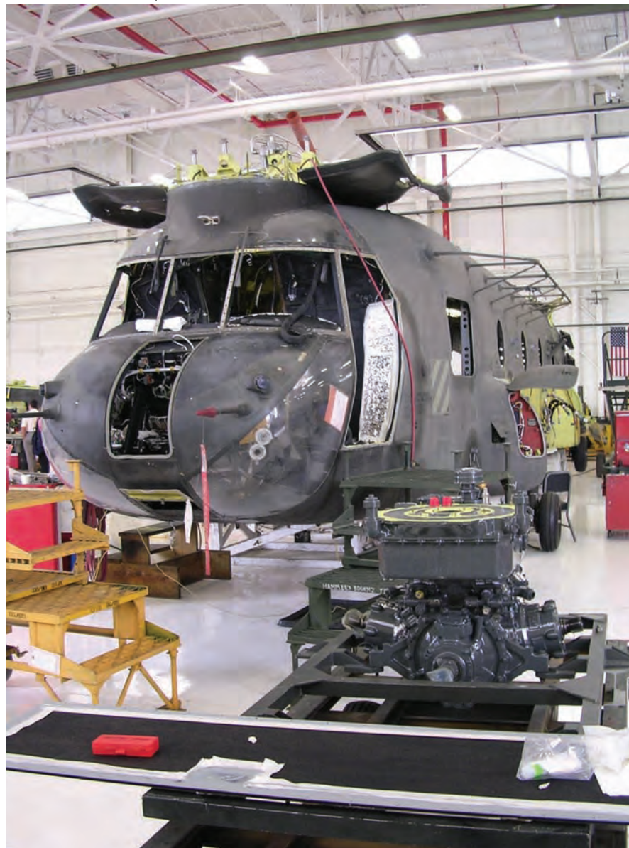
Aircraft have all major components repaired or replaced during Reset.
