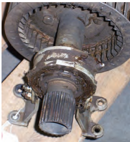
An OH-58 Oil Cooler Blower shows significant dirt, oil and contamination buildup upon disassembly.
