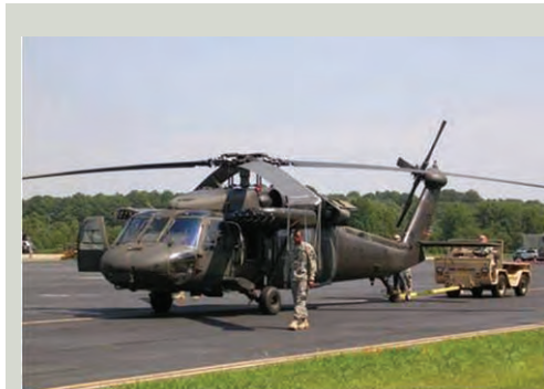
The Standard Aircraft Towing System (SATS) towing the UH-60.
