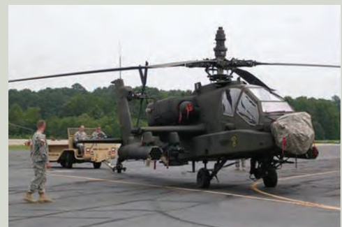
The Standard Aircraft Towing System (SATS) undergoes testing at Ft. Eustis towing an AH-64D.
