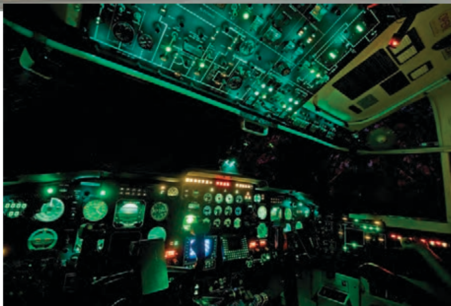
The C-23 Sherpa aircraft cockpits are receiving night vision goggle compatible modifications to provide tactical capability and safety for crew members flying night operations in combat and tactical airspace.
