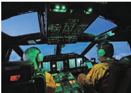
The C-27J Spartan's cockpit includes a state-of-the-art joint military communications suite and is compliant with Communication Navigation Surveillance and Air Traffic Management standards.
