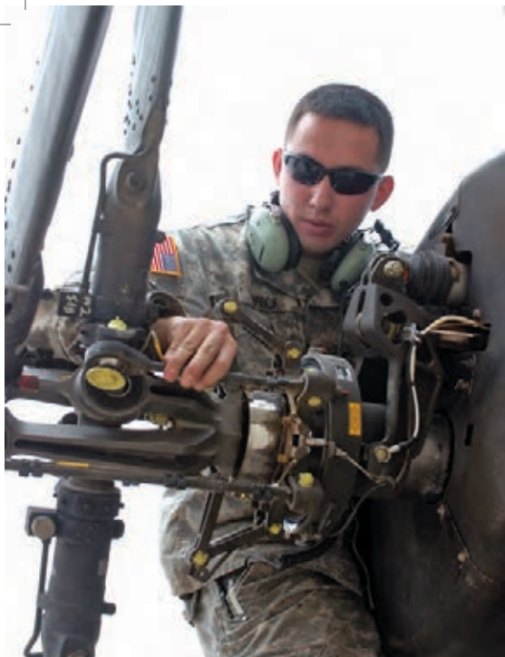
SGT Edmund Brock, an AH-64D aircraft mechanic performs service checks on the tail rotor assembly section of a Longbow attack helicopter.
