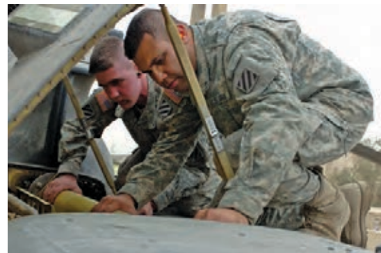
CH-47D aircraft mechanic PFC Thomas J. Nash, left, and phase team leader SPC Ruben D. Frias, both with Co. B, inspect the drive shaft on a Chinook helicopter.
