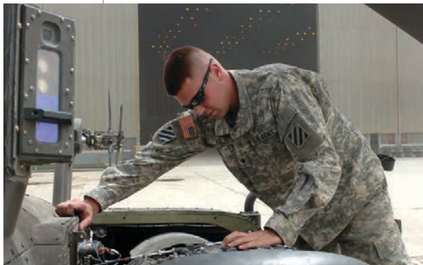
SPC Joseph A. Volz, an aircraft mechanic with Co. B, 603rd ASB, performs a pre-flight check on one of the 701C engines of an AH-64D Longbow attack helicopter.
