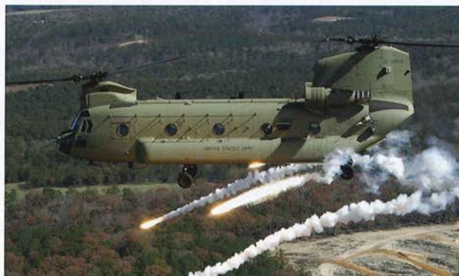
A CH-47 Chinook fires a combination of chaff and flare countermeasures during a systems test mission.
