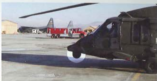
The AN/AAQ-22 forward looking infrared (FLIR) system, mounted up under the nose of the aircraft cockpit, is helping aircrews fly and locate people under difficult circumstances and high risk situations.
