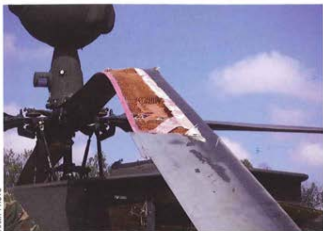
The damaged OH-58D Kiowa Warrior main rotor blade; the quick reaction of the crew saved their lives and the aircraft.
