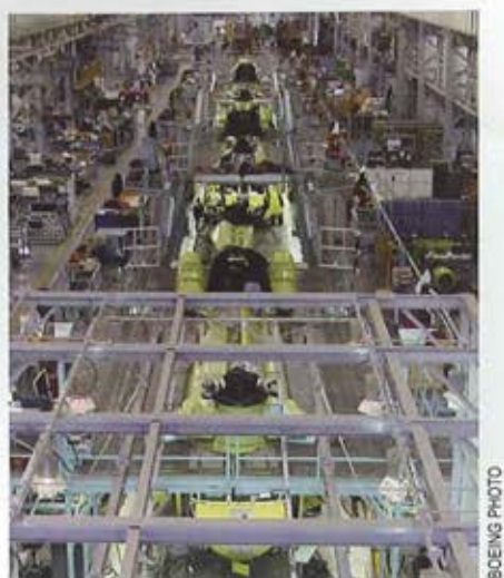
New build CH-47 Chinooks move down the assembly line at the Boeing Rotorcraft Systems facility in Ridley Park, Pa.
