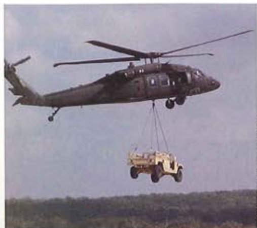
As part of the operational test, pilots from 4th Sdqn., 3rd Arm. Cav. Regt., conducted a variety of operational missions, including external loads such as lifting this humvee.
