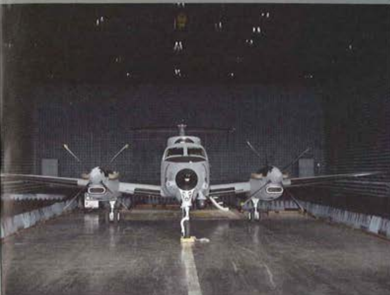
Above: An RC-12Q with the DASR during testing in the anechoic chamber.
