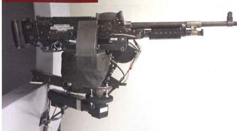
Figure 3: A key component of the NCMT is the realistic replica of the M240H weapon system which provides the feel and operational functionality of the actual aircraft machinegun.
