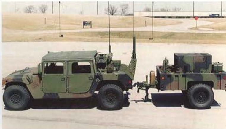
**The Tactical Terminal Control System provides initial air traffic services at remote landing sites.**
