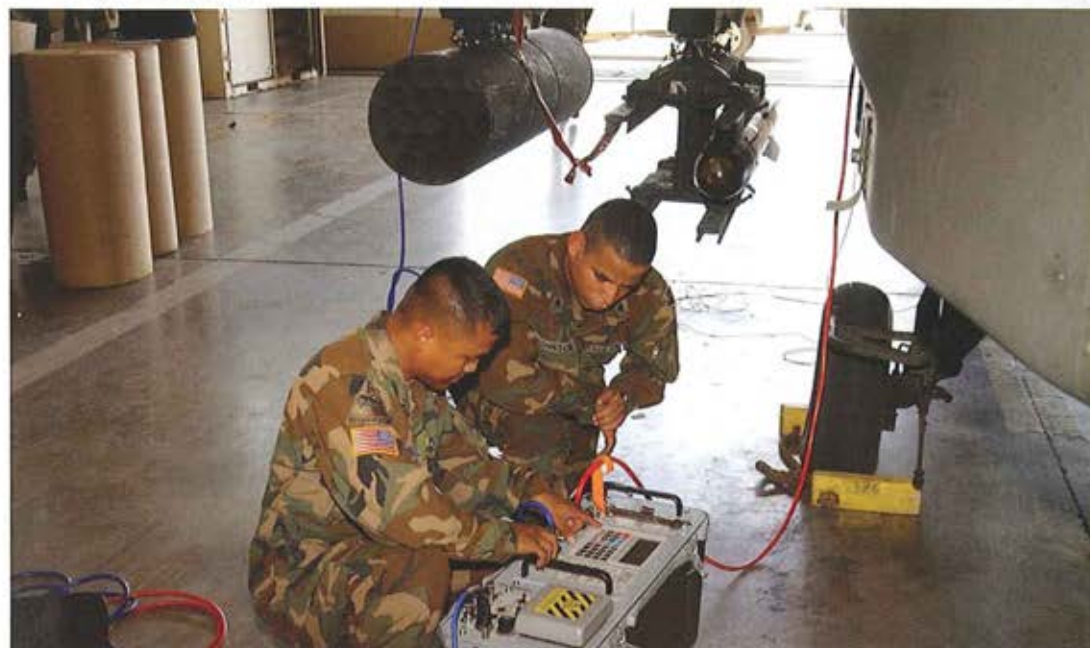
SSG Gernel Domingo shows SPC Timothy Johnson, both with 1st Bn., 4th Avn. Regt., how to calibrate the altimeter and speed indicator on an AH-64D Longbow Apache aircraft. Their unit has benefited from additional support personnel and equipment in the "Iron Eagles" transition to a combat aviation brigade.
