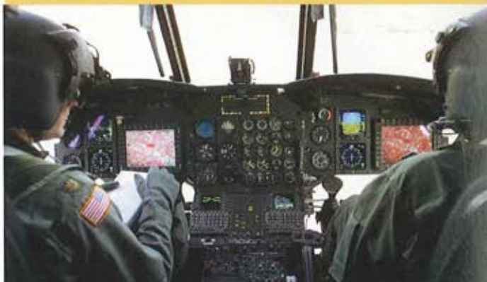
Above: In this prototype CH-47F cockpit, pilots have the opportunity to use multi-functional displays and other electronic gages which will be used to make the new CH-47F a fully 'glass' cockpit.
