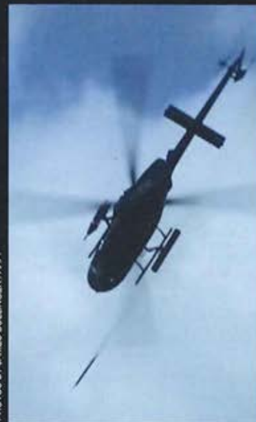
A rocket briefly illuminates an AH-64D firing at night. An OH-58D employs a rocket during a diving fire maneuver. The 2.75-inch (70mm) rocket is standard ground attack munition in use by Army attack and recon aircraft.
