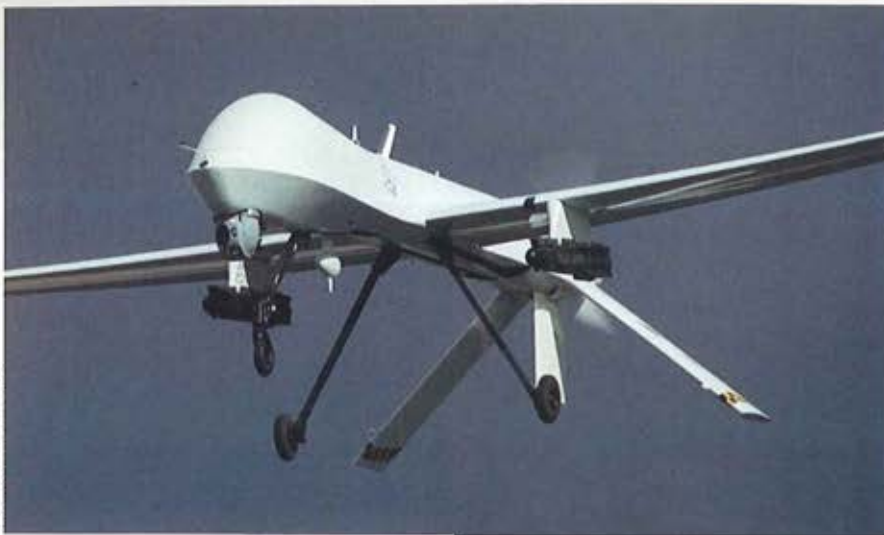
The P model HELLFIRE missile (a K model with modifications) mounted on the Predator unmanned aerial vehicle.
