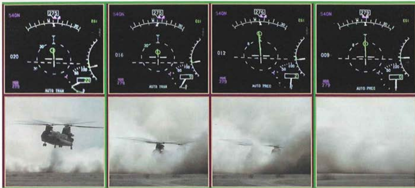
The brown-out situational awareness upgrade (BSAU) provides pilots with landing cues to safely land aircraft in brown or white out situations. Here the system is demonstrated with a CH-47 aircraft landing with the BSAU assist in a series of shots.
