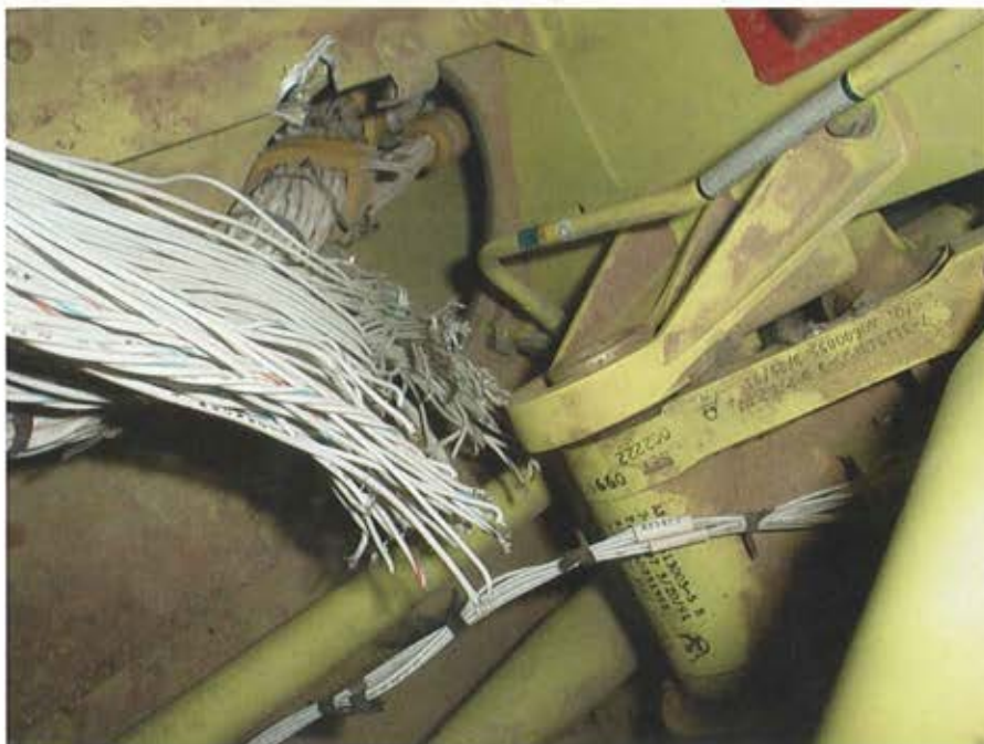
Shrapnel, small arms and machine gun fire can damage or sever wire bundles. Here an AH-64 Apache has combat damage to a wire bundle.
