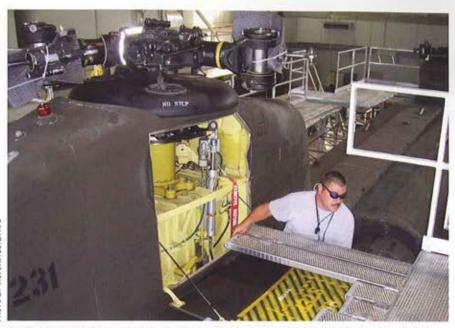
Mechanic David Ferguson sets adjustable platforms on the fall protection scaffold system prior to working on a CH-47 rotorhead.
