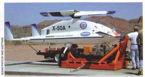
The X-50A Canard Rotor/Wing Dragonfly is one of several unmanned aerial vehicle initiates The Boeing Company is developing.
