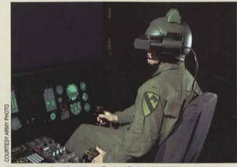
The Aviation Combined Arms Tactical Trainer (AVCATT) is an industryenabled mobile simulator system providing enhanced collective training for aircrews to operate together in a variety of virtual mission scenarios.
