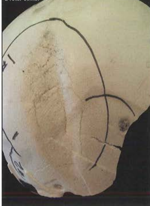
Figure 2. Helmet energy-absorbing liner permanently deformed following a rotor strike.
