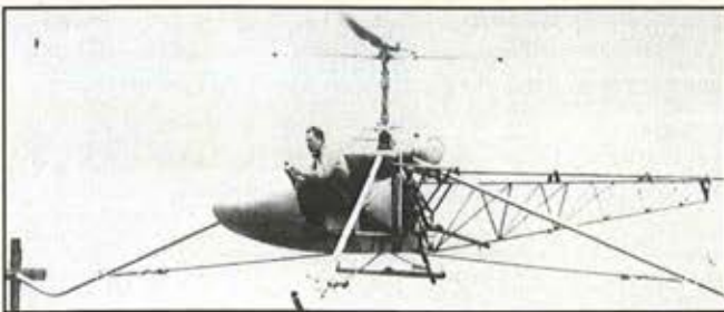
Arthur Young in free flight in Ship 1 (also known as the Model 30 and "Genevieve") in 1943. The first Bell machine had four long legs and no wheels in order to prevent the machine from inadvertently tipping over during initial hover testing. Young taught himself to fly while tethered to the ground in this machine. (Courtesy Bell Helicopter)
