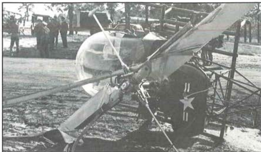
While there were no deaths or serious injuries during the program, there were several accidents and incidents. This overloaded H-13 crashed at Fort Rucker on Jan. 21, 1958, just before a firing demonstration.
