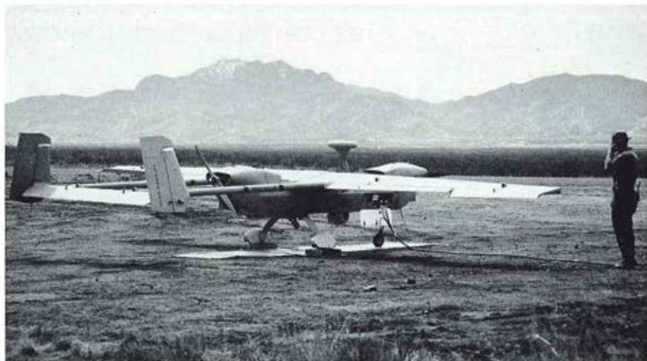
Above: The Pioneer UAV provides near-real-time Reconnaissance, Surveillance, Target Acquisition (RSTA), Battle Damage Assessment (BDA), and battlefield management within line of sight of a ground control station, both day and night.
