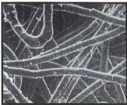
Random fiber structure of FNC plates enhances temperature, mechanical, and electrical performance
