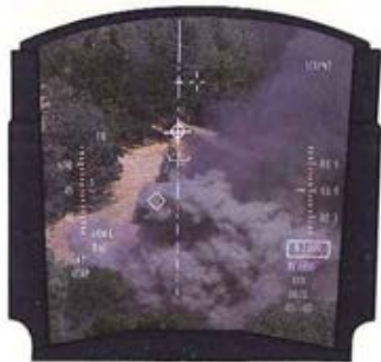
ATHS provides data for such HUD symbols as target LD, range and steerpoint.
