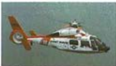
The Panther team is currently integrating the T800 engine into a U.S. Coast Guard HH65, a derivative of the Dauphin helicopter.
