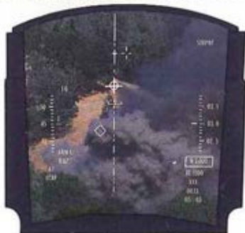
ATHS provides data for such HUD symbols as target ID, range and steering point.
