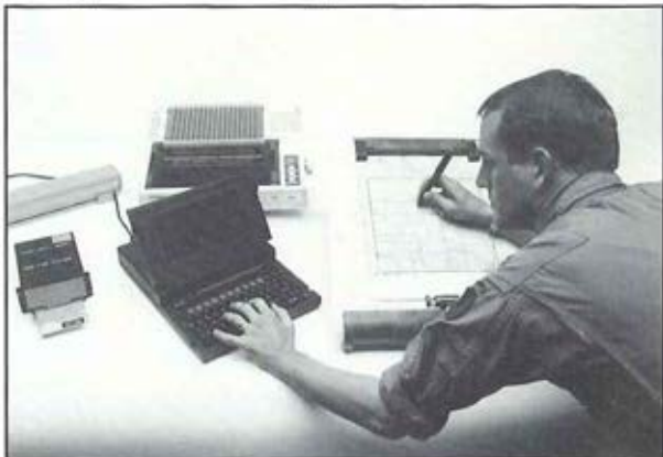
Pilot uses a map digitizer to input Flight Plan Information to the program.
