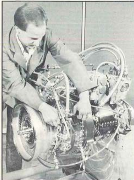
LEFT: Final arrangements being made to an Avco Lycoming/Pratt & Whitney T-800-APW-800 engine prior to testing.
