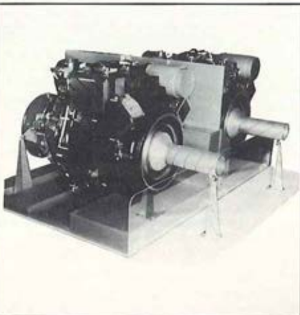
BELOW: The LHTEC (Allison/Garrett) T800 engine in a generic air vehicle mockup of twin T800 compartment in support of advanced installation studies.
