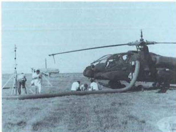
TOXIC TESTING — An AH-64A APACHE from the Aviation Development Test Activity undergoes the tests at Dugway Proving Ground, Utah to determine possible degradation of the helicopter operations in a toxic environment.
