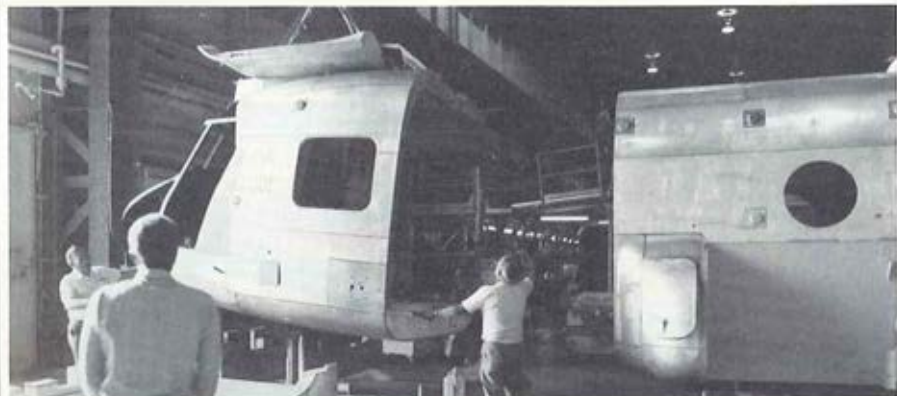
A NICE SPLICE — Splicing of the first all-new production model CH-47D for an international military customer, the Japanese Self-Defense Forces, occurred at the Boeing Vertol plant in Philadelphia earlier
