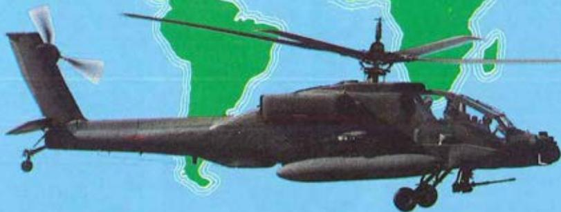
Ready for battle, the U.S. Army's AH-64 Apache can fly for 1,000 nautical miles into a 10-knot headwind with a 20-minute fuel reserve.
