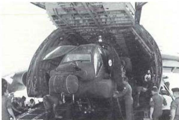
**SIX IN ONE** — APACHE helicopters were recently airlifted in a giant U.S. Air Force C-5A GALAXY transport for the first time ever in an operation designed to certify loading procedures for worldwide
