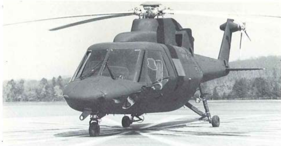
ABOVE: The Sikorsky-ACAP helicopter with its all-composite airframe. BELOW: SHADOW, the Sikorsky-funded experimental research aircraft - a single-pilot cockpit attached to the nose of an S-76 helicopter.
