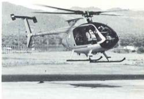
The Hughes Advanced Rotor Project (HARP) is shown on its maiden flight on April 23, 1985. The HARP uses a modified Hughes 530F for the testing of all composite rotor blades.
