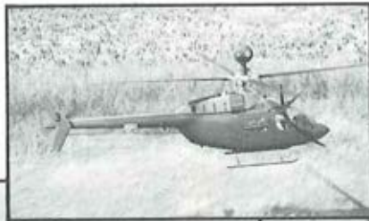
BELOW: Kiowa with inflatable floats.
