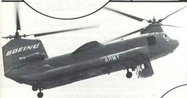
ABOVE: The fly-by-wire, triple hook CH-47 with the craft operated from the retractable load controller crewmember's (LCC) station. CIRCLE ABOVE: The Boeing Model 347 — the world's largest tandem rotor 'copter with a controllable tilt-wing.
