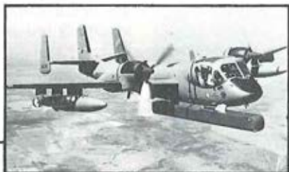
LEFT: OV-1 Mohawk equipped with SLAR
