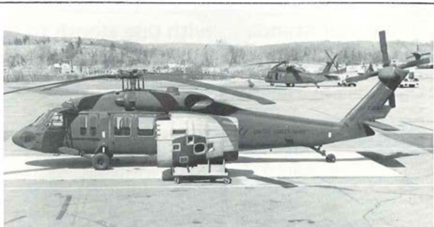
NEW BLACK HAWK FUSELAGE — A lighter, less expensive Composite Rear Fuselage (CRF) with far fewer detail parts and fasteners than the standard metal rear fuselage is being developed for the UH-
