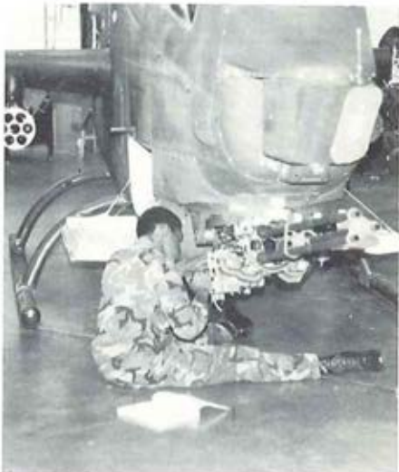
CLOCKWISE FROM UPPER LEFT: INSTALLING AN AH-1 TAIL ROTOR; REPAIRING THE AH-1S 20MM GUN'S UNIVERSAL TURRET; CHECKING A CH-47 MAIN LANDING GEAR STRUT; CHECKING A UH-60'S TAIL ROTOR DRIVE SHAFT.
