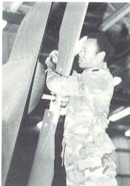
CLOCKWISE FROM UPPER LEFT: INSTALLING AN AH-1 TAIL ROTOR; REPAIRING THE AH-1S 20MM GUN'S UNIVERSAL TURRET; CHECKING A CH-47 MAIN LANDING GEAR STRUT; CHECKING A UH-60'S TAIL ROTOR DRIVE SHAFT.
