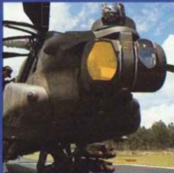
TADS/PNVS; weapon delivery, navigation system.
