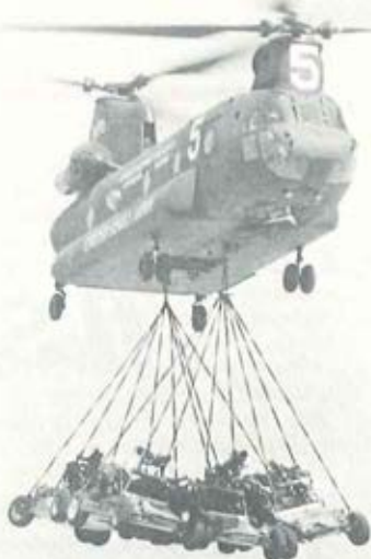
THE "D" CAN LIFT SEVEN DUNE BUGGIES/FAST ATTACK VEHICLES (FAV'S), ONE INTERNALLY, SIX EXTERNALLY, AND 14 PAX.
