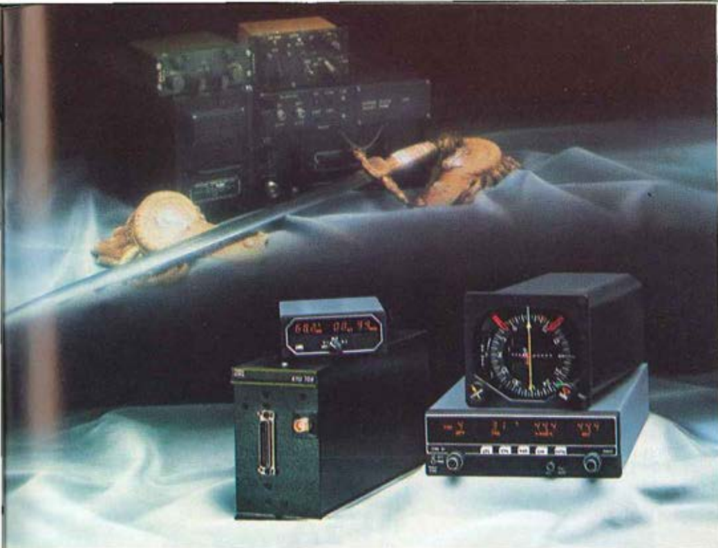
A totally integrated VOR/LOC/GS and 10-waypoint RNAV computer system, 252-channel TACAN system and a Slaved Horizontal Situation Indicator
