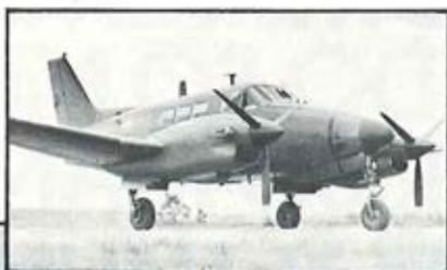
BELOW: An RU-21D with SEMA antenna array similar to that on an RU-21E reconnaissance aircraft.
