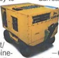
support cart which is sling-transportable by the UH-1H. Ready for production, the AGPU, powered by the Model 36 gas turbine, provides pneumatic, AC, DC, and hydraulic power for ground checkout or starting. In addition, it is self-propelled for helicopter towing.
