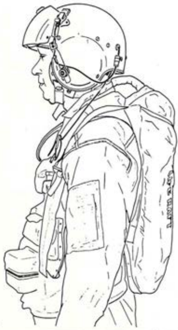
FIGURE 2 —The new back-mounted, lightweight flotation kit that will provide increased water survivability in both arctic and tropical climates.
