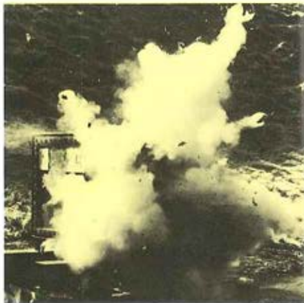
FIG. 2B—IMPACT APPEARANCE—TEST WITH POWDER-FILLED STRUCTURE
