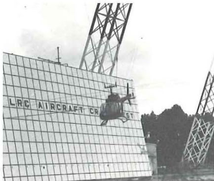
FIG. 4—Langley Research Center test sequence with OH-58 Kiowa in the bottom of its pendulum arc cuts multiple wires simultaneously.
