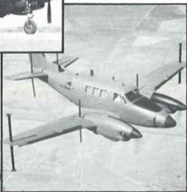
BELOW: An RU-21D with SEMA antenna array similar to that on an RU-21E reconnaissance aircraft.
