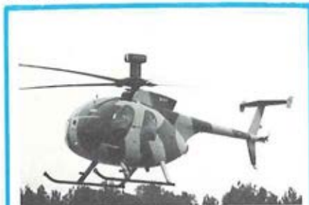
HUNTER-KILLER — A one-of-a-kind aircraft, a Hughes Helicopters 500MD sports a Mast Mounted Sight made by Martin Marietta. A company-funded project, the ship visited USAAVNC.
