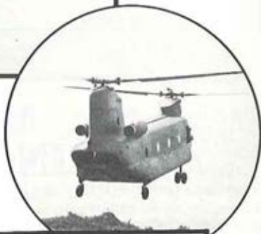
ABOVE: The fly-by-wire, triple hook CH-47 with the craft operated from the retractable load controller crewmember's (LCC) station. CIRCLE ABOVE: The Boeing Model 347 — the world's largest tandem rotor 'copter with a controllable tilt-wing.
