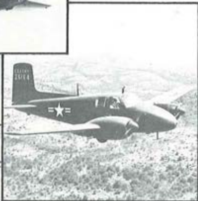
LEFT: RU-8D with APS-85 Radar
