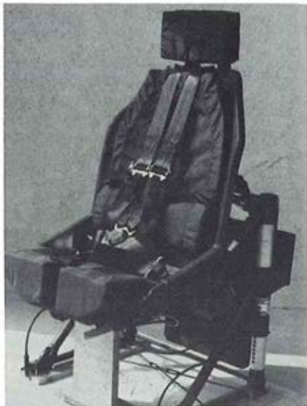
FIGURE 2—The armored crash attenuated pilot/copilot seat undergoing final qualification.
