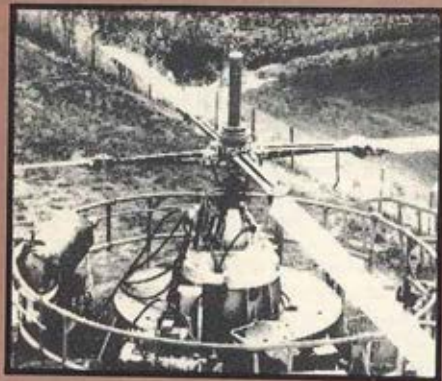
FIGURE 2—The Bearingless Main Rotor (BMR) which promises to reduce the number of parts in a four-bladed rotor hub assembly from 400 parts to approximately 60.
