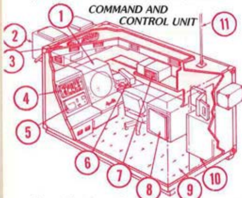
A partial cutaway of a command and control master unit to be tested. 1) Display and control station. 2) Climate control unit. 3) Air distribution. 4) Cartridge magnetic tape unit. 5) Command & response unit. 6) Keyboard printer. 7) Radio mtg provisions. 8) Power control. 9) AN/UJK computers; Not shown. 10) AN/UJK-7 computer. 11) Radio antenna.
