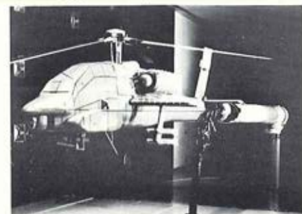
FIGURE 1 — The YAH-64 V/STOL Wind Tunnel Research Model is shown undergoing hub/pylon drag investigations and evaluation of the relocated horizontal tail. The tests, undertaken at the Langley Research Center, employ design models that have the capability of testing the fuselage and rotor system of each of the Army's current inventory of single rotor helicopters.
