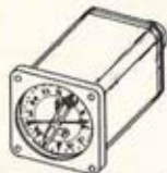
Radio Magnetic Indicator
