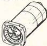
Triple Torque Indicator
