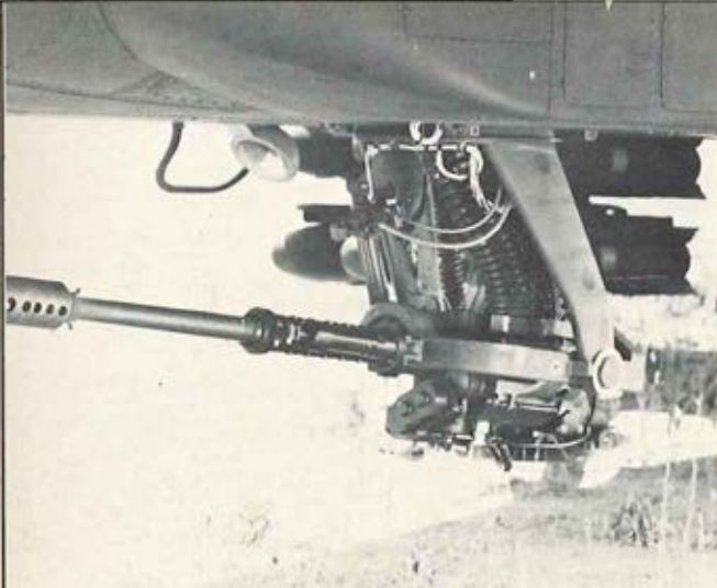
30mm Chain Gun was tested during the AAH Fire Control Survey.
