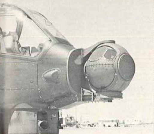
Top Left: The Integrated Helmet and Display Sight System (IHADSS). Top Right: The Martin-Marietta PNVIS as installed on a test YAH-64. Bottom Right: Northrop Corp.'s Pilot's Night Vision System (PNVIS). Bottom Left: The Airborne Target Acquisition Fire Control System (ATAFCS).
