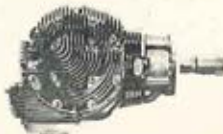
Engine Nose Gearbox
